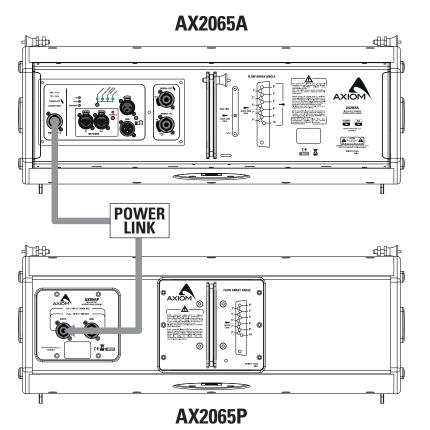
The DA module employed for powering the AX2065A delivers in an ultra-compact package a maximum power of 2000W. Moreover, each AX2065A is able to power an additional passive AX2065P module through the available power output on the back panel. This feature will allow to assemble very competitive system solutions both for rental and installation applications.
